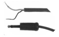
D. Peel back the outside piece of wire surrounding the inner coated wire.
